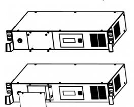
4 Pull on the white tag on the battery and remove the battery from the unit.
