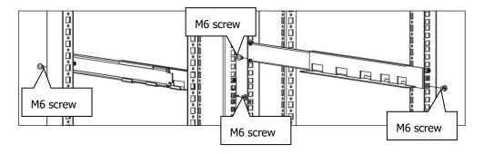
**Step 3:** According to the UPS height, insert 6 nuts in the proper location.
