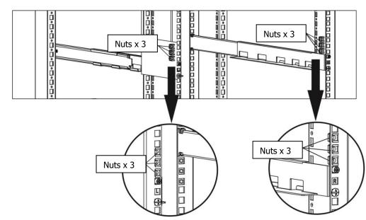
**Step 4:** Place the UPS with assembled ears on the rail support.
