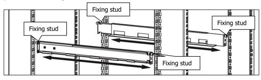
**Step 2:** Use the 4 x M6 screws to mount rail sliders into the chassis. See chart below:
