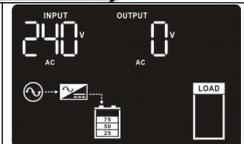
**Step 2:** Press and hold the "Select" button for 3 seconds to enter Setting mode.
