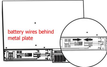
Battery wires are connected behind metal plate. Connect the AC input.
