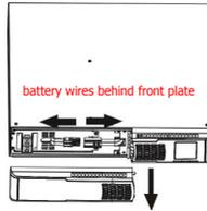
Remove the screws on front plate and remove plate. Disconnect battery wires.
