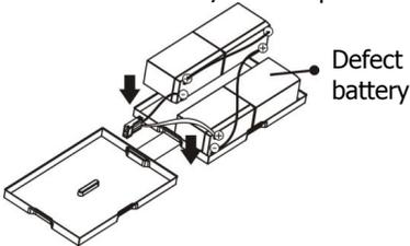
Step 4: Cover the other side of plastic shell as below chart. Then, battery kit is assembly well.
