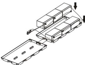
Step 4: Cover the other side of the plastic shell as shown below so that the battery kit assembly is ready for installation.
