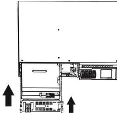
Slide the battery box back in the original location, re-connect the battery wires and fasten the screws on metal cover securely.
