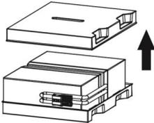
Remove the top cover of battery box and replace the batteries inside.
