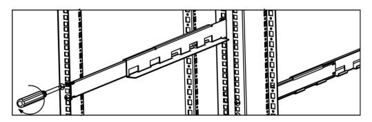
**Step 3:** According to UPS height, put nuts on proper location.
