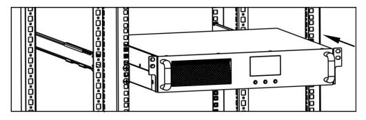
**Step 5:** Fix the UPS in position with screws
