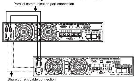
Diagram 2: Wiring diagram of parallel system
