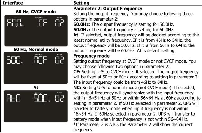
Note: If the UPS is set to CVCF mode, the bypass function will be disabled automatically. But when a single UPS without parallel function is powered on with mains and before the UPS finished the startup, there will be a few seconds of voltage pulse (same as the input voltage) on the bypass output. If you need to remove the pulse on this mode to protect your load
