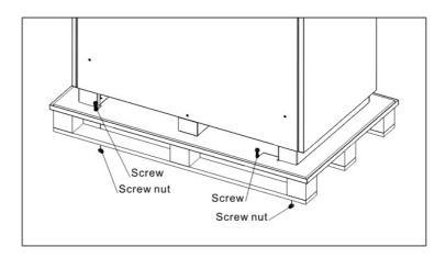
(4) Use a crane or other tool to remove the cabinet from the pallet and place the battery cabinet.
