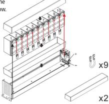
6. Assemble the top cover and lock the screws in sequence.
