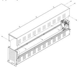
5. Assemble the 9AH 12V battery into the empty battery module, as shown below.
