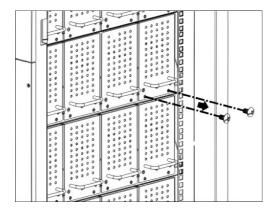
3. Remove the empty battery module.
