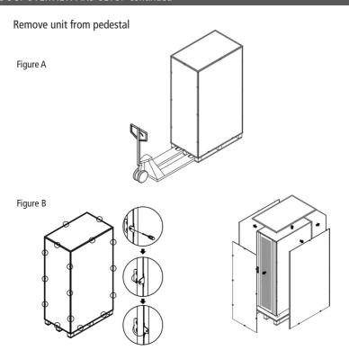
(3) The four sides of the battery cabinet feet are fixed with screws and nuts. Loosen the screws and nuts to remove the fixing on the cabinet and pallet. Refer to figure below.
