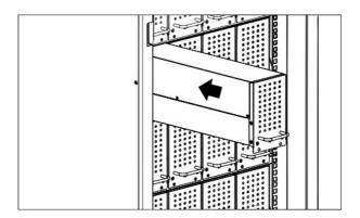
8. Fasten screws to lock the battery modules.
