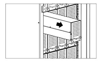
4. Remove the empty battery module cover.
