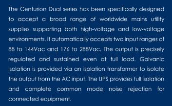
The Centurion is designed to protect critical computer, communications, industrial, medical and other mission critical equipment. A true online double conversion UPS, the Centurian is designed to guarantee trouble free operation of protected equipment in any harsh electrical environment. Versatile management and hardware options offer the flexibility to build up a power protection solution to fit any application.
