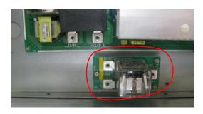
Step 5: Connect the OP Relay board to the PSDR board with two short wires, and make the brown wire that removed in step 3 cross the yellow core 5 turns, connect the brown and blue wire to the OP Relay board refer to the following picture, connect the 4 pins brown cable from OP Relay board to PSDR
