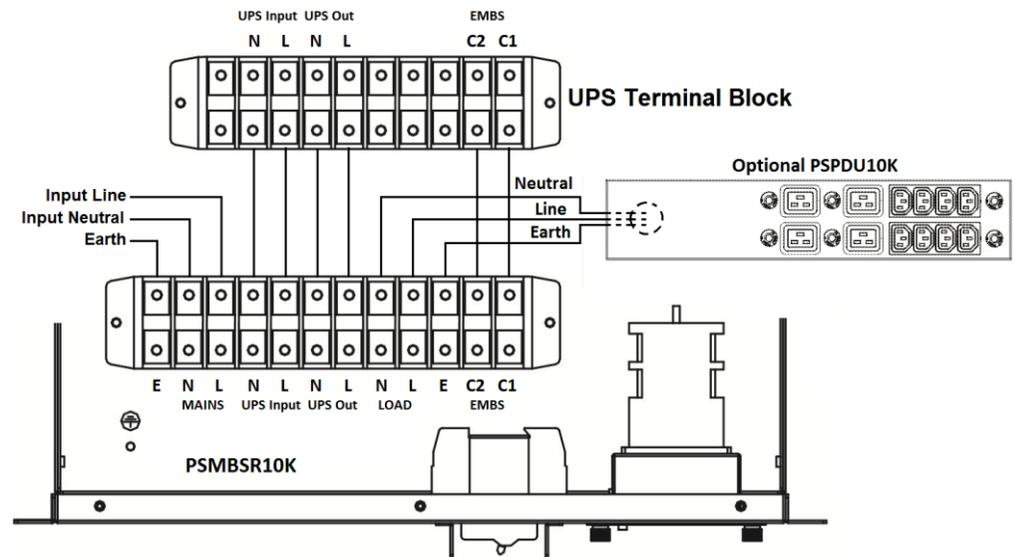
**WARNING:** It is essential to connect the EMBS (C1, C2) terminals on the UPS to the EMBS (C1, C2) terminals on the PSMBSR10K (Maintenance Bypass Switch module). Failure to do so will cause damage to the UPS and void the warranty. Check the UPS model User manual for the rear panel UPS Terminal Block pin assignment.
