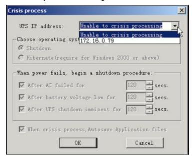
After selecting the UPS network card IP address (SNMP Lite IP address), you can set the crisis management for the server.
