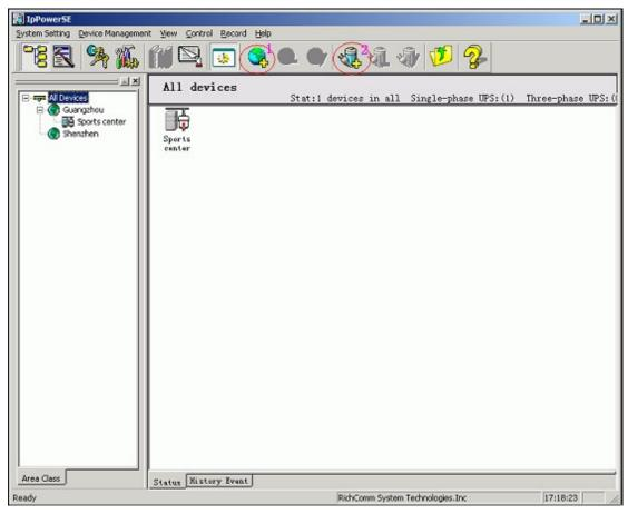
Press the button marked 1 shown in the above page to divide the area. If there is little device data to be divided or no need for dividing area press button 2 to add device directly. The Add Area is shown below:
