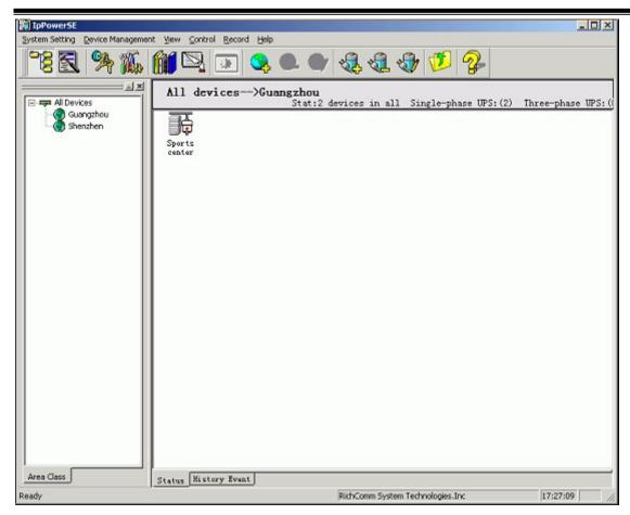
Choose a certain device in the navigator and press the right button in the mouse. Choose the "Device Status" and the main window will display the status graphic of the current device, as below:
