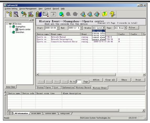
9.3 View system log. Users can view the user operation when logged in the monitoring system. It offers inquiry filter, information output in Excel and print functions.
