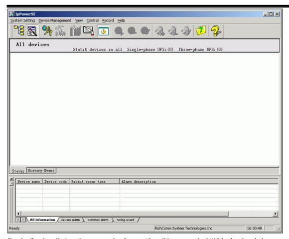
For the first installation please press the shortcut "keys" button marked "1" in the chart below to logging in before you are authorized to add and modify any device. IP Power SE defaults to have a vacant password.
