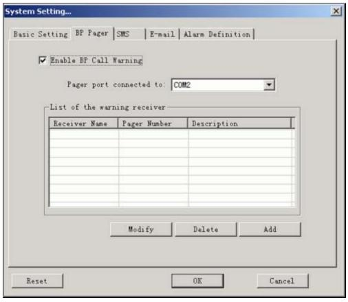
To add the BP Warning Receiver, please press the "Add" button shown on the above page, input the Receiver name and BP number. After the adding users can choose to "Modify" or "Delete" the added receivers.
