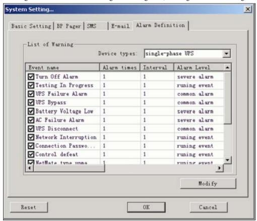
Double press the warning information to be modified. If an alarm needs to be continuously broadcast without the confirmation of the administrator, you can choose the option "warning untill it's canceled or confirmed" and set the interval time for voice broadcasting. You can also
