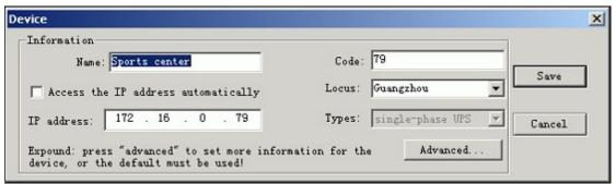
Input device "Name", "Number" and "IP Address" and then select the type for the device to be monitored. The device type must be accordant to the one with NetmateII. For adding more information please press "Advance" to enter the advanced configuration page.
