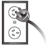
3 NEVER Connect a laser printer / scanner to the UPS outlets. This may cause damage to the unit. The, following type of equipment may cause some problems because the battery output mode of this unit is not sinusoidal; Inverter, Transformer, AC line filters and PFC power supplies.
