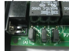
Fig. 6 Jumper setting for ACTIVE CLOSE
