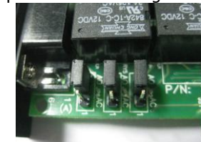
Fig. 7 Jumper setting for ACTIVE OPEN
